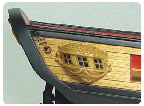
**Photo 7.** The stained quarter badge placed on the model of the brig *Syren*. Four coats of stain on the Super Sculpey matched the color of the planking well.
