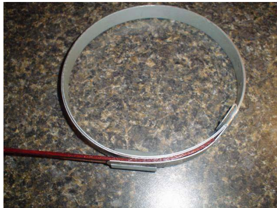
Figure 3. – Plank Steaming Jig.
