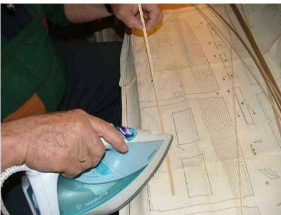
Figure 1. – Applying the Steam iron to a Strip.
