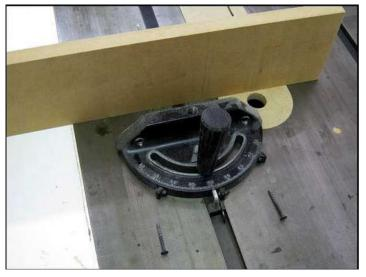
The addition is nothing more then an auxiliary fence from a piece of 3/4" thick MDF or good quality plywood attached with screws thru the reverse side of the gauge. Cut a piece of MDF about 4" tall and 18 to 24" long. Drill pilot holes for on the backside for the wood screws.
