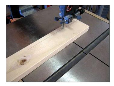
Draw a pencil line on a test piece of lumber exactly parallel to the edge. Start the band saw and freehand cut along the line. When you are cutting straight on the line, stop feeding the work piece into the blade and hold the board down on the saw table firmly by hand and shut the saw off. Let it wind down to a stop.
