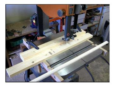
Run the stock through the blade at a slow, steady feed rate. Let the blade do the cutting. It will cut straight and true each and every time.
