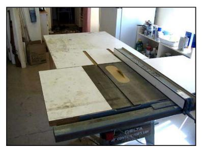
While it's true that most stock rip fences that are provided with table saws are notorious for being frustrating at best, I wouldn't recommend you running out and buying an aftermarket fence just yet. For one thing they are expensive and second with a bit of adjustment and care taken in its use the one you have may prove to be adequate for your needs.
