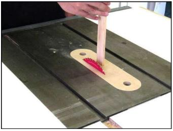
Hold the throat plate blank down tightly with a stick. Turn on the saw and slowly raise the blade to cut through the plate.
