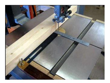
For a rip fence, use any nice straight length of board. Use the setting on the adjustable bevel to set the fence while measuring the thickness of the cut you want from the blade.
