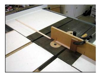
After returning the empty miter gauge to the in-feed side of the saw blade, butt the end of the off-cut piece up against the stop block and repeat the process, continue until the stock is gone.
