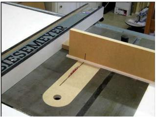
Slide the miter gauge with the stock forward, leaving the block behind.
