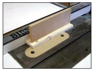
Push shoes are designed to be expendable, but if being used correctly, they should not get chewed up that fast. If you have to replace them frequently, that's an indication you are attempting to cut pieces that are to thin, which requires setting the blade a little too close to the rip fence. Basically your finished piece is on the wrong side of the saw blade, and you should be using a alternate method of cutting them instead, See the section on using the "rip fence stop" later in this article.
