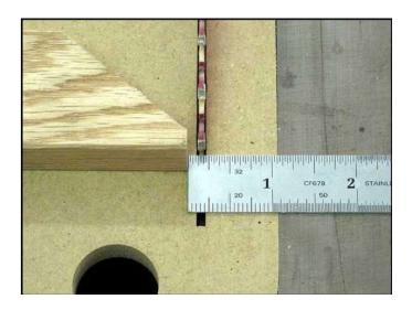
Let's get in for a close look. Make sure the tip of the fence stop is 3/32" from the blade. When it's set tighten the lock nut.
