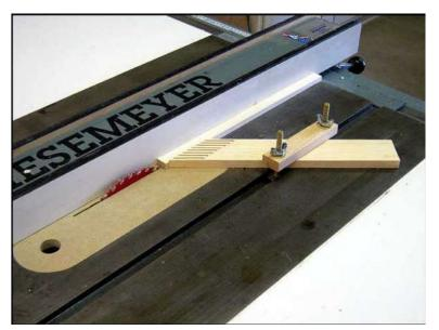
The next step is to cut the 3/8" x 3/4" strip into 1/4" widths. Set the fence to 1/4" and clamp a feather board to the saw table.
