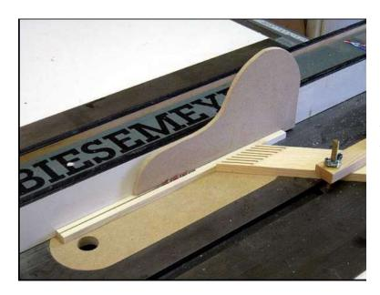
Use the push shoe to guide the stock trough the blade.
