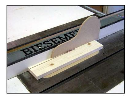
Set the table saw fence to 3/8". That will be the first cut. Use a push shoe to guide the stock through the blade.
