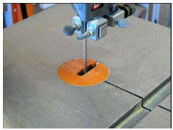
This will not work. It's not flush with the saw table and the gap around the saw blade is too wide. Change it out with a zero clearance throat plate made from 1/8" hardboard or Masonite. Cut a little slot and drop it in.
