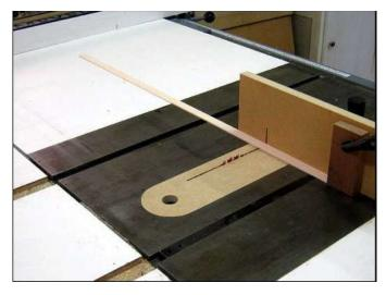
Slide the miter gauge forward all the way through the blade. Keeping yourself clear of the saw blade move the off-cut piece out of the way. Remove the keeper piece with the miter gauge still forward. Don't try to slide the miter gauge back with the keeper piece still in place against the stop block.
