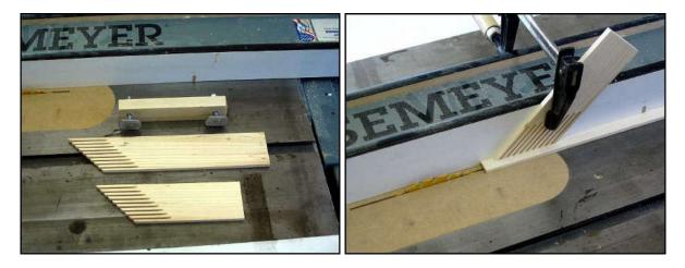
The longer feather board gets clamped to the surface of the saw table. Its job is to hold the stock against the surface of the rip fence. The hold down clamp is made from a block of wood, two standard toilet bolts, two washers, and either two wing or hex nuts. The bolt heads are cut to fit the "T" slot on the saw table. Here's how the feather board clamps to the table. Just a heads-up tip, not all table saws have T-slot miter gauge slots.
