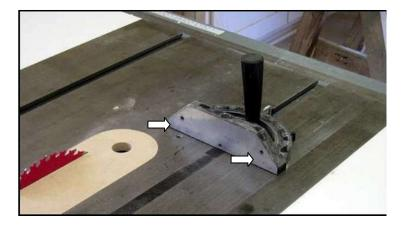
The next modification is to the miter gauge. The miter gauge is heavily used for cross cuts to length after the stock is cut to thickness and width.
