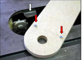
On the underside of the plate, drill and countersink for some #6 or #8, half-inch long flat head wood screws. Locate these screws so they act as little "footies" (red arrows) against the throat plate ledge in the saw table (white arrow).
