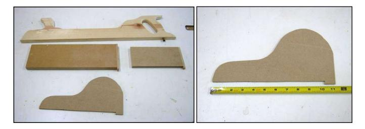
Push shoes are about 12" long and 6" tall. They are made from 1/4" thick hardboard or tempered Masonite.
