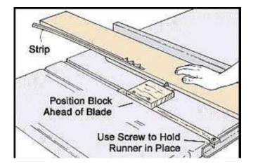
One solution to this problem is the jig shown above right. It's just a block screwed to a runner that sits in the saw's miter gauge slot.
