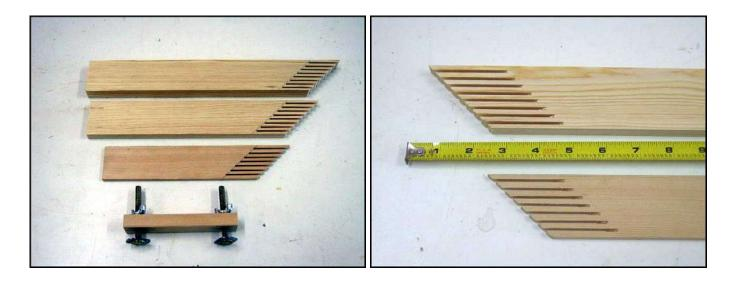
I find it handy to have pairs of feather boards in three levels of thickness 1/4", 1/2", & 3/4". In the photograph on the left, the one at the top is 3/4" thick pine, 2" wide, and 12" long, the middle one is 1/2" thick, and the bottom one is 1/4" thick. The angle of the end is 45 degrees. The fingers are 1/8" wide, while the slots are a saw kerf in width. Use the feather boards that most closely match the thickness of the stock being cut.
