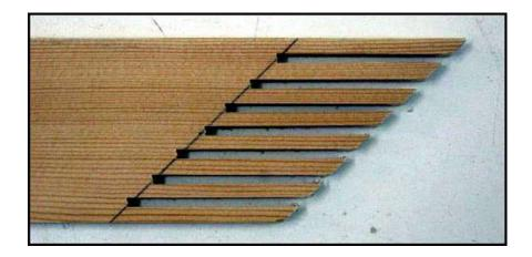
I always make the feather boards in pairs; one long and one short (see image on the left). The short one is clamped to the rip fence (see image on the right), so it doesn't protrude too much and get in your way when cutting, causing an unsafe condition. Its job is to hold the stock down against the saw table surface.
