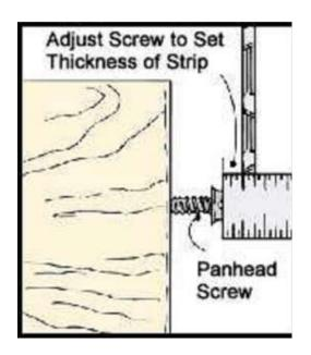
Setting the jig is easy. Position it alongside the blade and fine tune the jig by turning a pan head screw driven into one edge, see the drawing at right. Then pull the jig back so it sits ahead of the blade. Now butt your work piece against the screw and lock the rip fence against the work piece. Make a cutting pass, then repeat the process on each additional pass. All the strips will be the exact same thickness."
