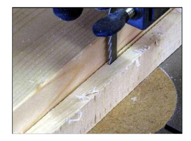
How thin can you cut on a band saw? How about 1/16"
