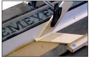
The next accessory we need is a rip fence stop. The fence stop assists in accurately setting the saw fence to cut thin strips. There are a number of plans available for these, from simple too complex. Simple is better. The fence stop drops into the miter slot on the table saw. Here are the parts and the fence stop in use:
