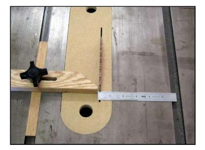
Do the 3/32" thickness cut first. That's a close cut, too close to try to set the saw fence. Instead, use the rip fence stop attachment we made earlier. Drop the fence stop into the table saw miter slot and loosen the lock nut. Adjust the fence stop so the tip is 3/32" outside the blade. Note, the saw teeth have a set to the right and left, so measure the 3/32" from the tip of the saw tooth that has its set toward the side that the fence stop is on, and not just to side of the saw blade.
