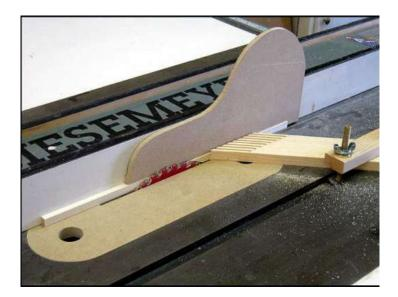
The first cut on the 3/4" wide strips leave about a 3/8" wide leftover. The leftovers can get a second cut at 1/4" width. Leave the saw fence set at 1/4". Adjust the feather board for the leftover piece and saw again.
