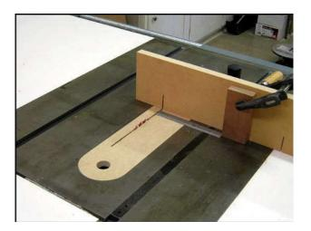
Butt a piece of stock tight up against the block. Make sure the rip fence is well out of the way so it won't interfere with the movement of the free end of the stock.
