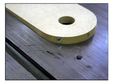
Adjust the foot screws in/out to ensure the throat plate is exactly flush with the table. Adjust the edge screws in/out to take up and left/ right or forward/back slop. You want the blank throat plate fitting stable and flush, yet easy to get in and out.
