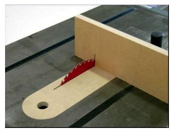
The auxiliary fence acts as a zero clearance throat plate by straddling the blade and giving good support to the work piece on both side of the cut. You can reposition the auxiliary fence left or right to suit your needs. As can be seen in the following picture my fence has been chewed up pretty good from use. When it's too far-gone, toss it and put on a new piece.
