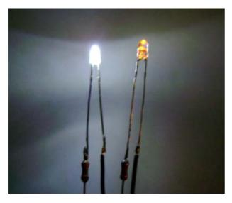
In the next picture you see the white and yellow LED's from the side, the yellow LED does not give out much light from the side. This is the disadvantage with LED's compared to light bulbs, light bulbs give out the same amount of light from all sides, the light from a LED comes mostly out of the domed top
