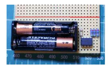
The three light board utilizing AAA cells installed in the model. The device will be cut from the breadboard along the red line. Finished dimension will be 1.125" X 2.75 or 29 X 70 mm. You must supply a two cell AAA battery holder. For more lights simply duplicate this layout.
